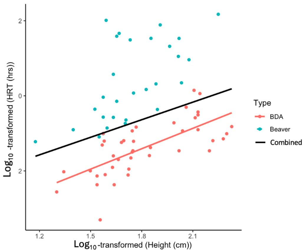
Figure 5. Scatter plot showing the relationship between Log<sub>10</sub>-transformed Height (cm) and Log<sub>10</sub>-transformed Hydraulic Residence Time (HRT) (hrs) for Beaver Dams (blue) and Beaver Dam Analogs (BDAs) (red) in semi-arid watersheds of Washington and Idaho, USA. The black line represents the combined regression line for both datasets and the red line represent the regression lines for BDAs.
