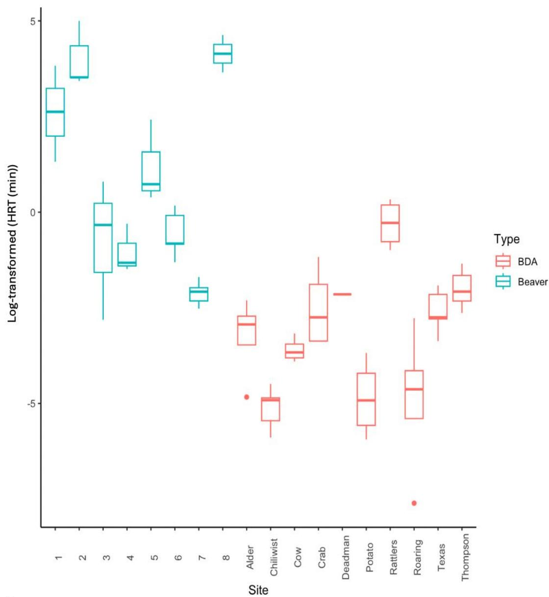
Figure. 4. Log-transformed mean ( $\pm$  se) of Hydraulic Residence times for each BDA and beaver dam site in semi-arid watersheds of Washington and Idaho, USA.
