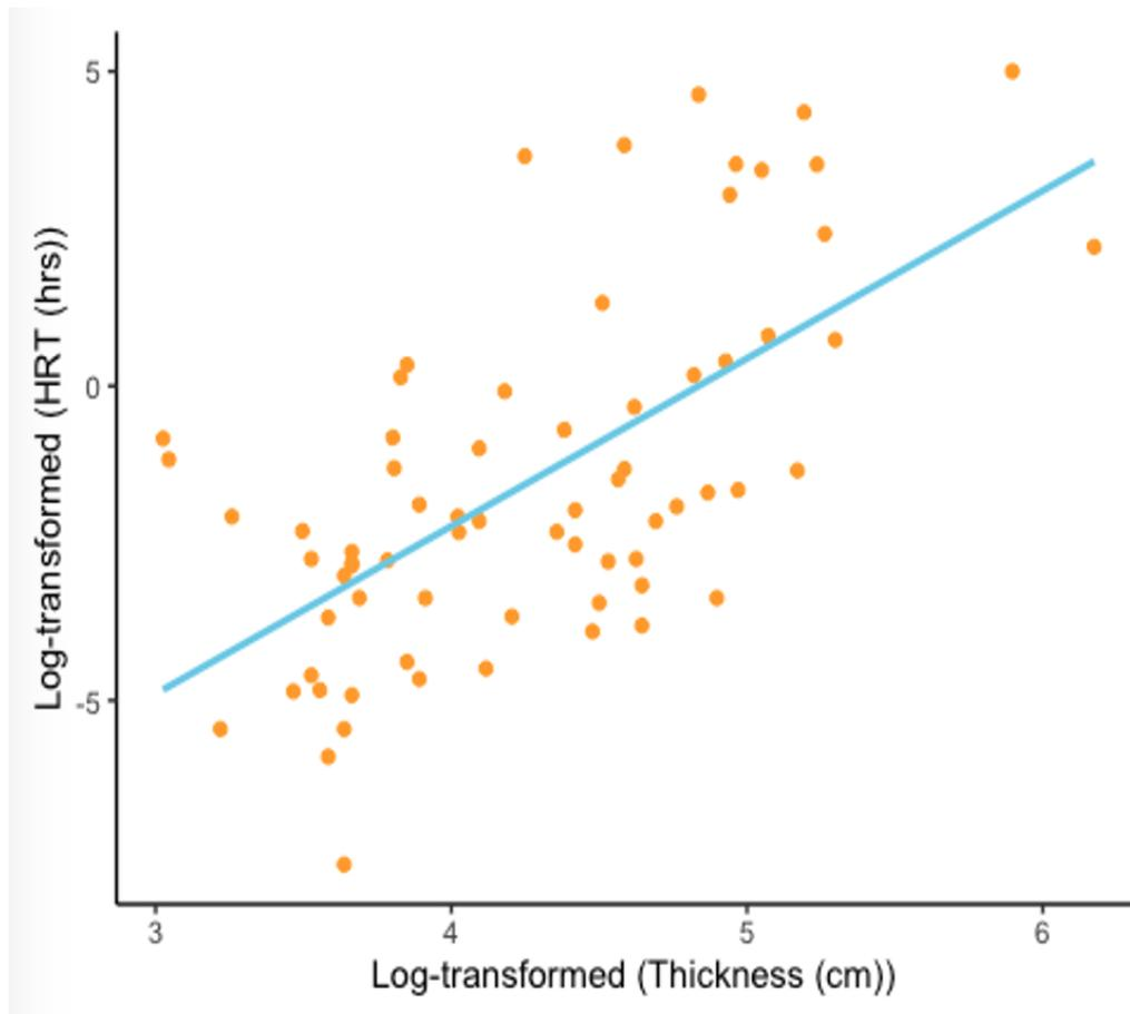
Figure 6. Scatter plot for both dam types showing the relationship between log-transformed hydraulic retention time and log-transformed dam thickness in semi-arid watersheds of Washington and Idaho, USA.
