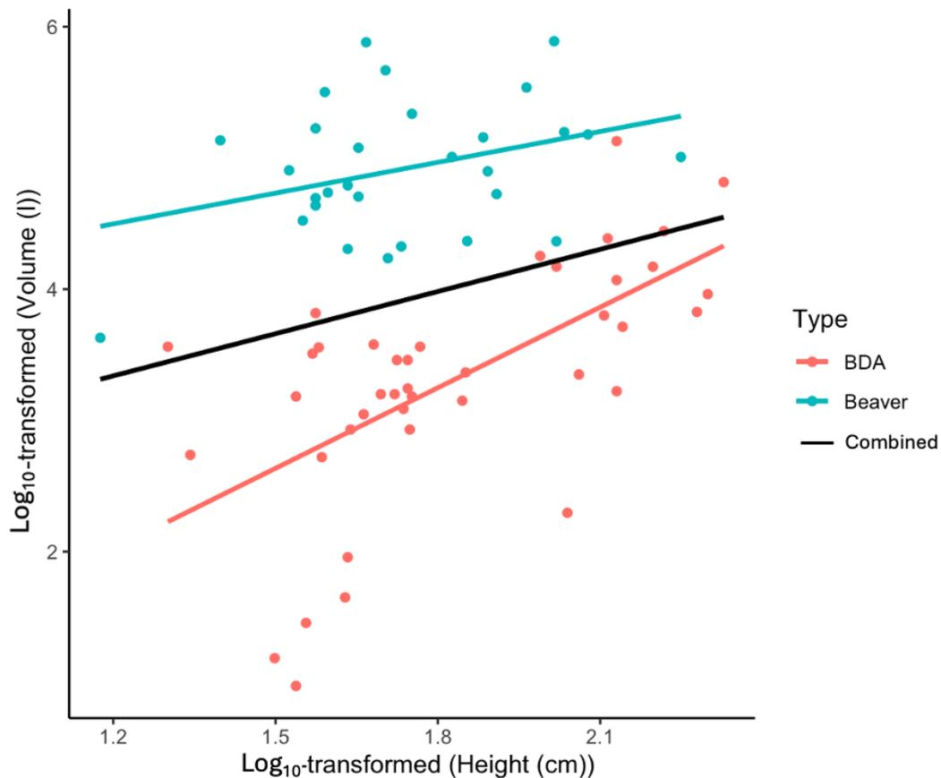
Figure 10. Scatter plot showing the relationship between Log<sub>10</sub>-transformed Height (cm) and Log<sub>10</sub>-transformed Volume(l) for Beaver Dams (blue) and Beaver Dam Analogs (BDAs) (red) in semi-arid watersheds of Washington and Idaho, USA. The black line represents the combined regression line for both datasets and the separate red and blue lines represent the regression lines for BDAs and beaver dams, respectively.
