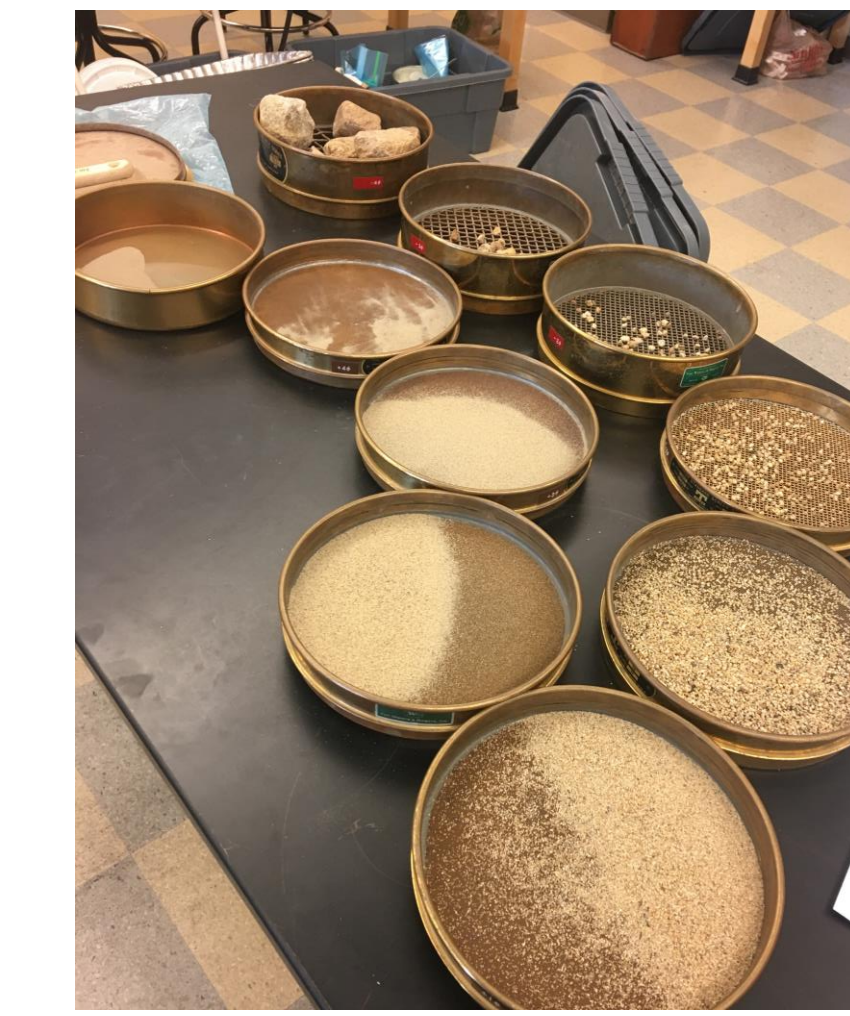
Fig. 9: Representative sample, showing the sieved streambed samples.
